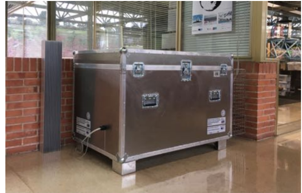
Fig. 2. aBox prototype. The development of this was essential for the design of the aluminum elements created to reduce the thermal bridge that guarantees the pressure between the heat sink and the TEM.
